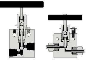
Pinned Stem Rolled Style Stem
