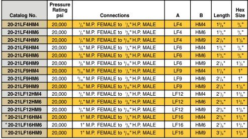
\* Can be rated to 30,000 psi if used with 1" O.D. x 7/16" I.D. tubing.
